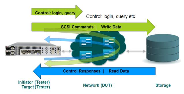
Illustration 2. Validating DCB-enabled data center switches with iSCSI deployment
