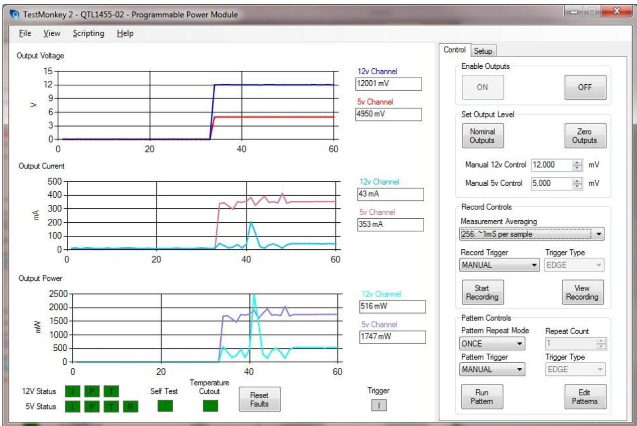
The graphs display data based on the current **Measurement Averaging** rate. By default there is no averaging, increasing this to average over 1mS greatly reduced the noise level that we see on the current and power graphs.
