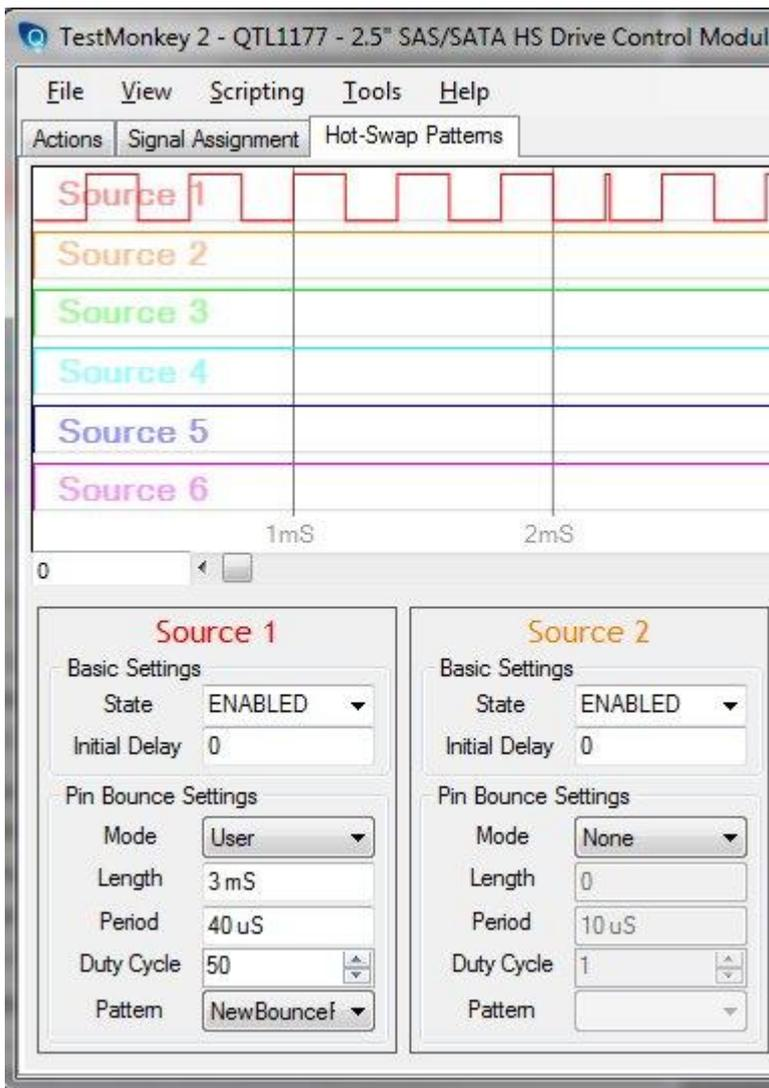
The new pattern is not shown on the timing display. The example pattern is another simple square wave but of a different frequency. The extra spike just after 2mS is the discontinuity at the end of the pattern.
