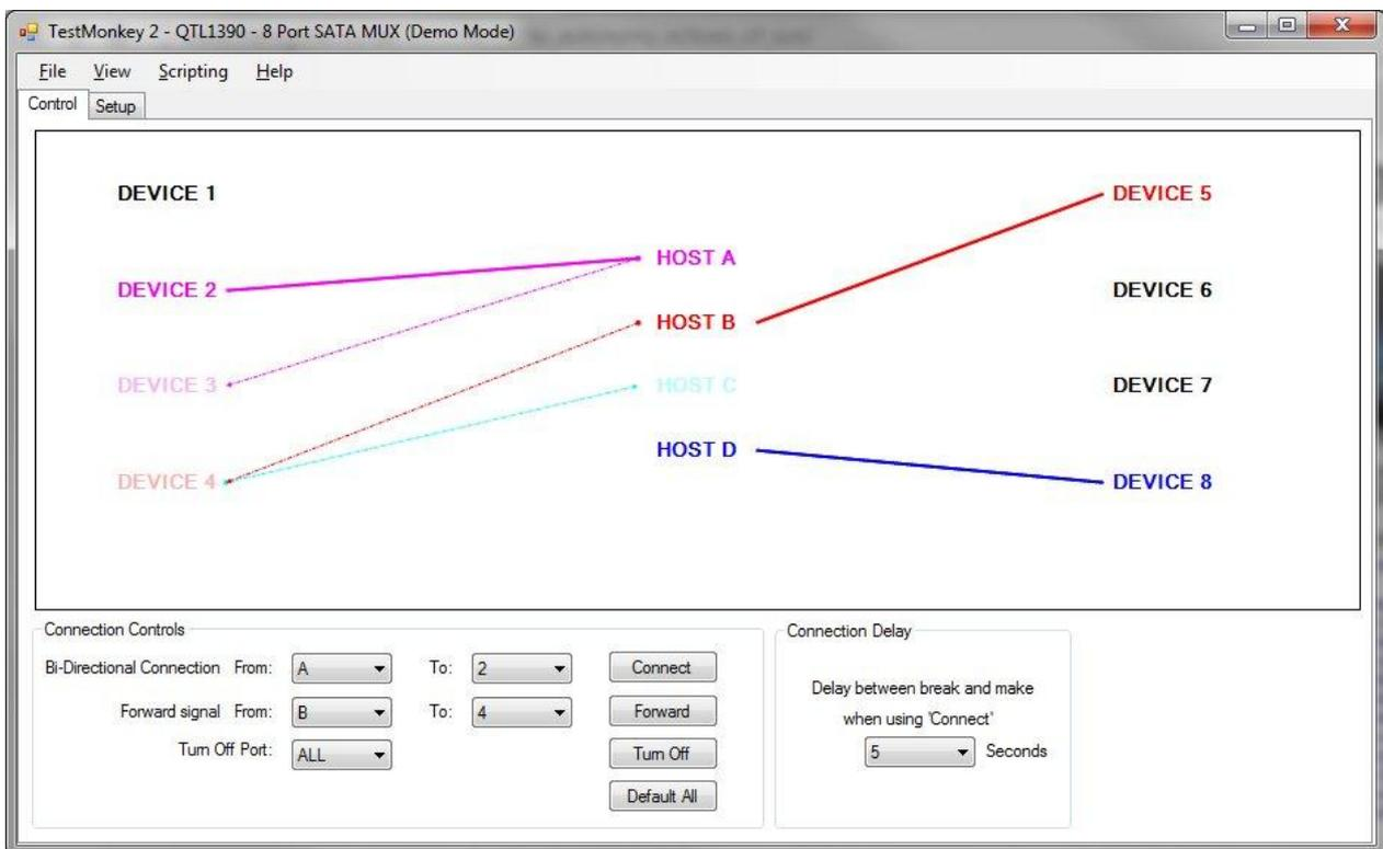
Unlike the 'Connect' command, the 'Forward' command does not automatically remove any related links. In this case the link from **4** to **C** has been left intact
