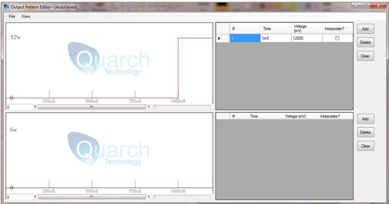
Edit the point so the output will be 12v after 10mS. The result of this action can be seen of the graph.
