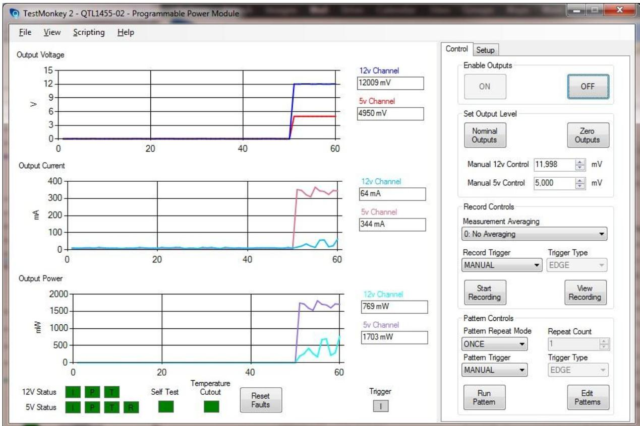
The voltage graph shows the increase in output voltage. In this case there is a disk drive attached to the PPM but it is not set to spin up.
