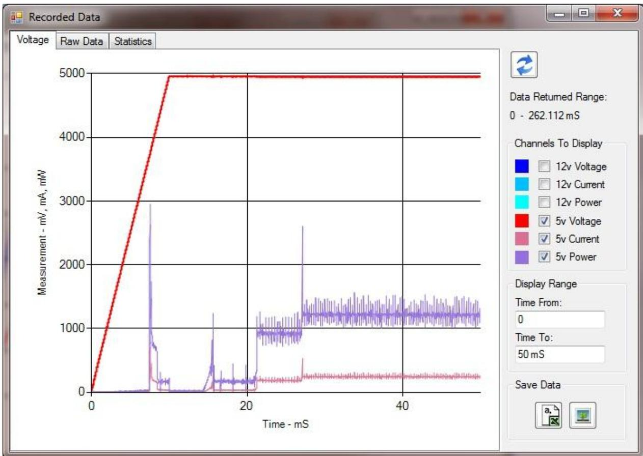
Looking only at the 5v channel, we can add the **power** and **current** selections and see that the drive does not pull much power until the 5v rail reaches over 3000mV
