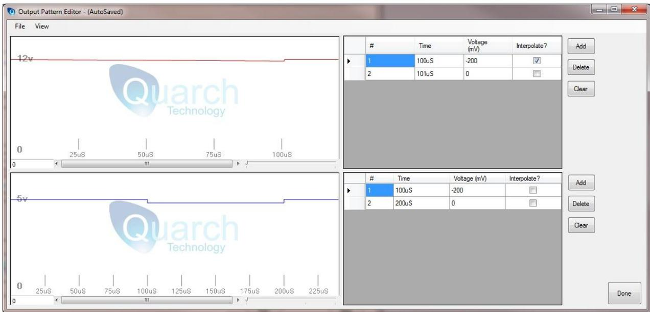
On the main control screen, we can set the **Pattern Repeat Mode** to **COUNT** and the. This means that the count value to 10. This will mean the pattern is repeated 10 times when **Pattern Run** is pressed.
