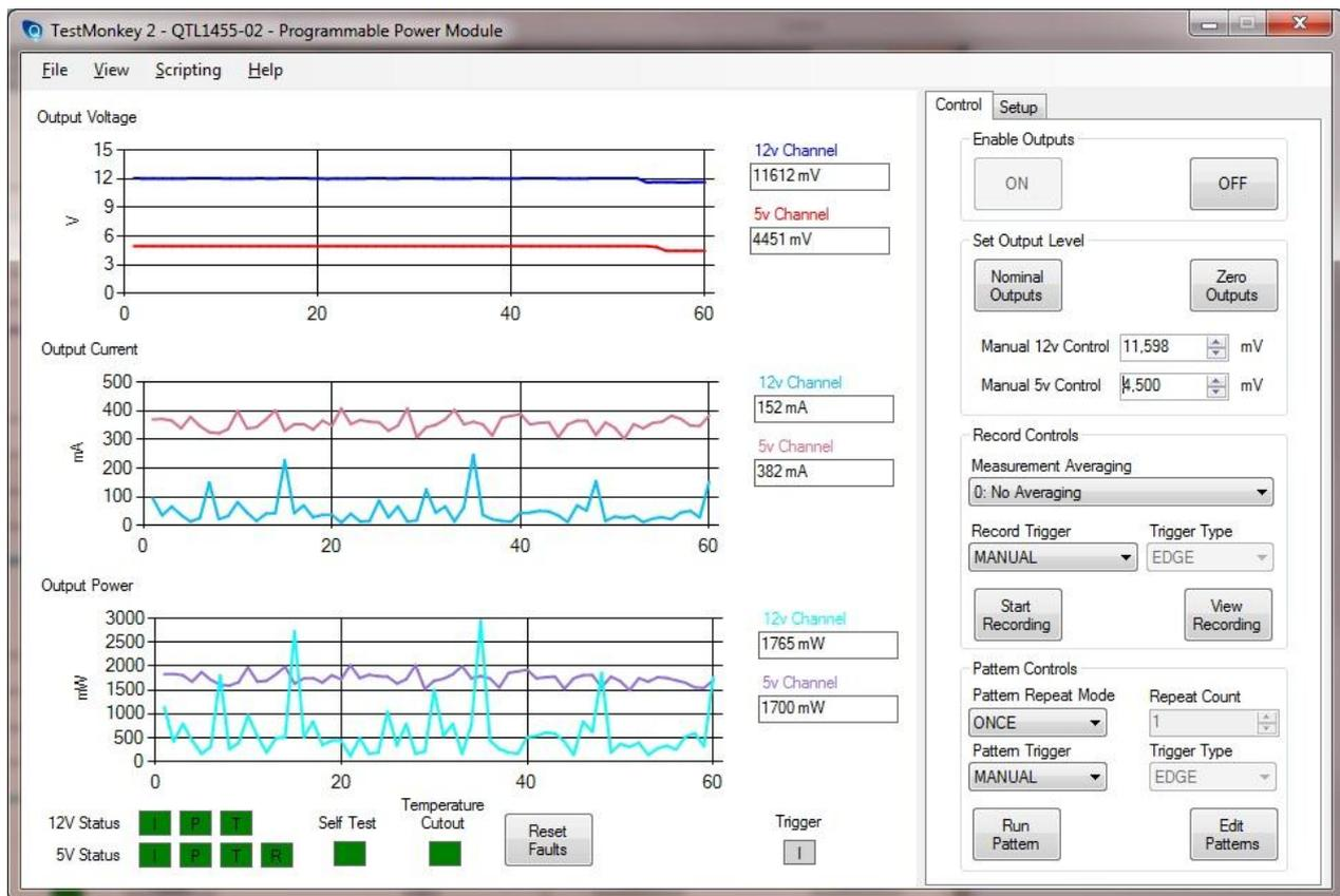
You can edit the output voltage level by editing the **Manual Control** boxes. Changes here will happen immediately (assuming the outputs are enabled).
