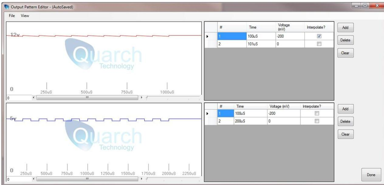
When the pattern repeat controls are altered, we see the effect this will have on the pattern editor. In this case, the 12v pattern is a sawtooth shape while the 5v pattern is a square wave.
