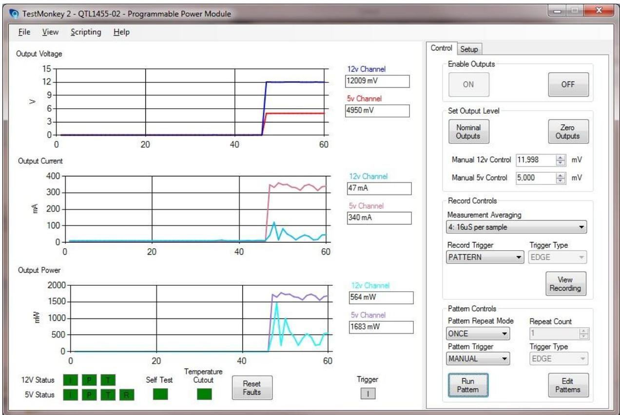
The effect of the pattern will be to ramp up the voltages, we can see this on the graphs as the attached device powers up. In this case, the pattern is set to **ONCE**. This is a transition pattern, so running it a second time would result in the output levels hitting the maximum output limits.
