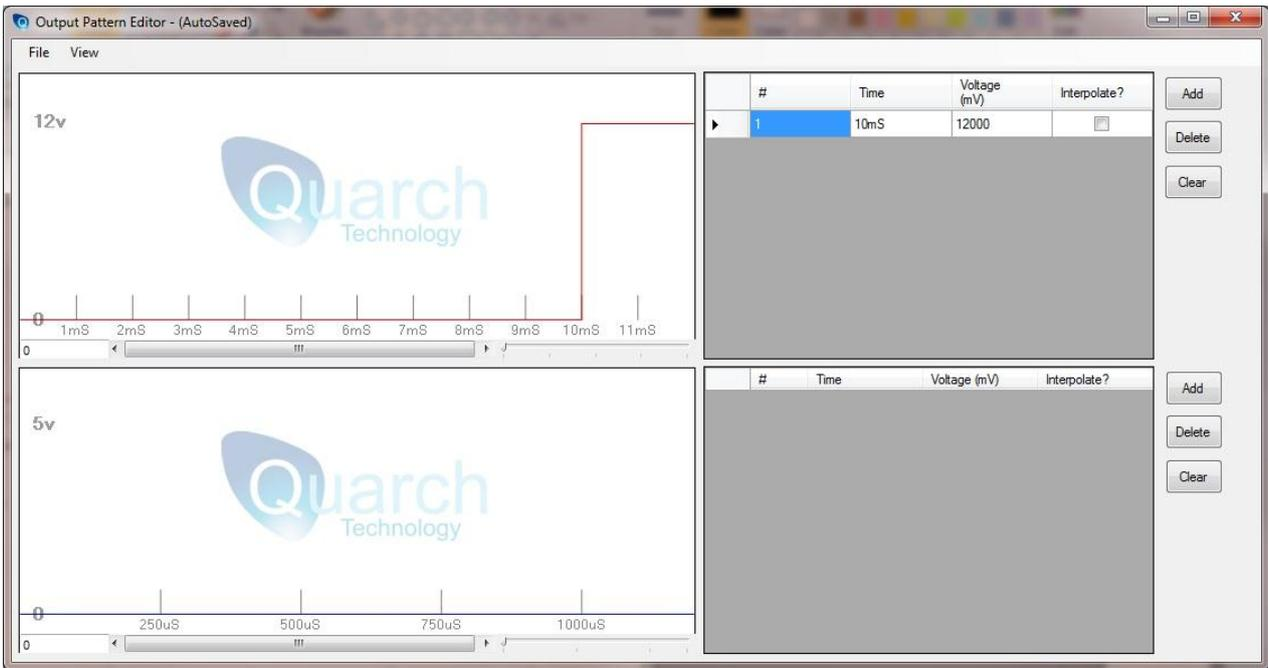
We want a ramp rather than a step, so select the **Interpolate** option so the output moves steadily up to the selected value over 10mS
