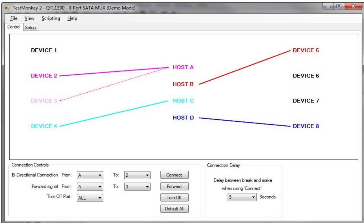
The dashed line indicates the forwarding link. The arrow head also shows the direction of the link.
