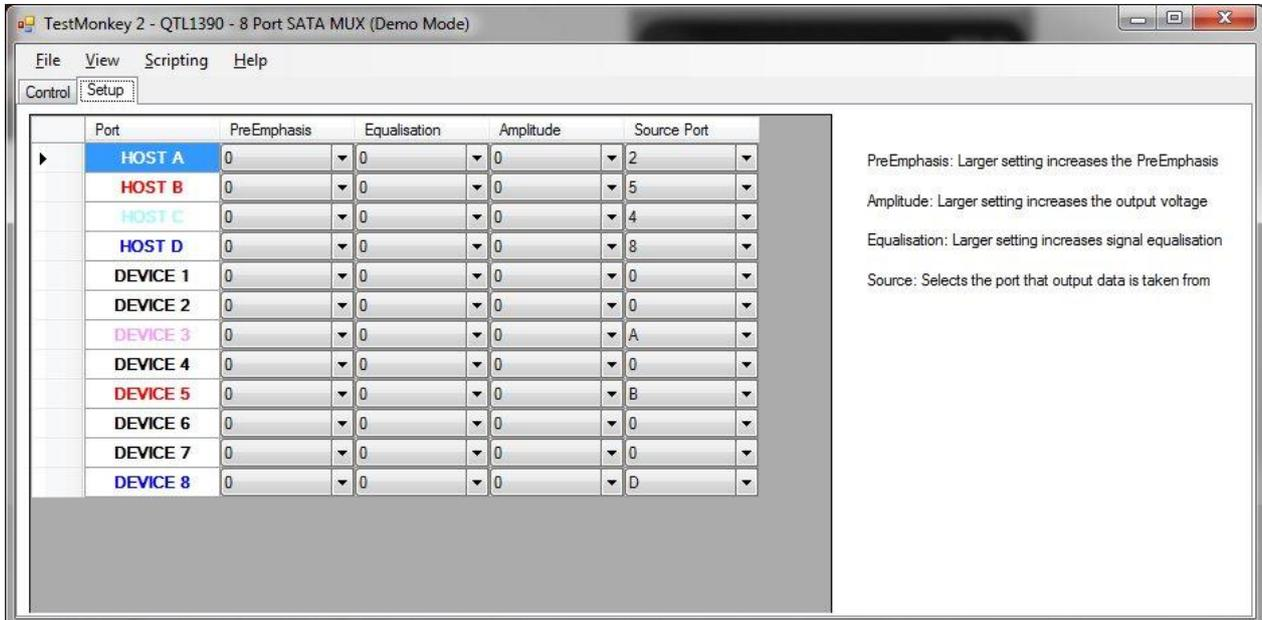
On the Mux setup page, you can select the value to use for each port. See the technical manual for the module for details on the affects of these settings.
