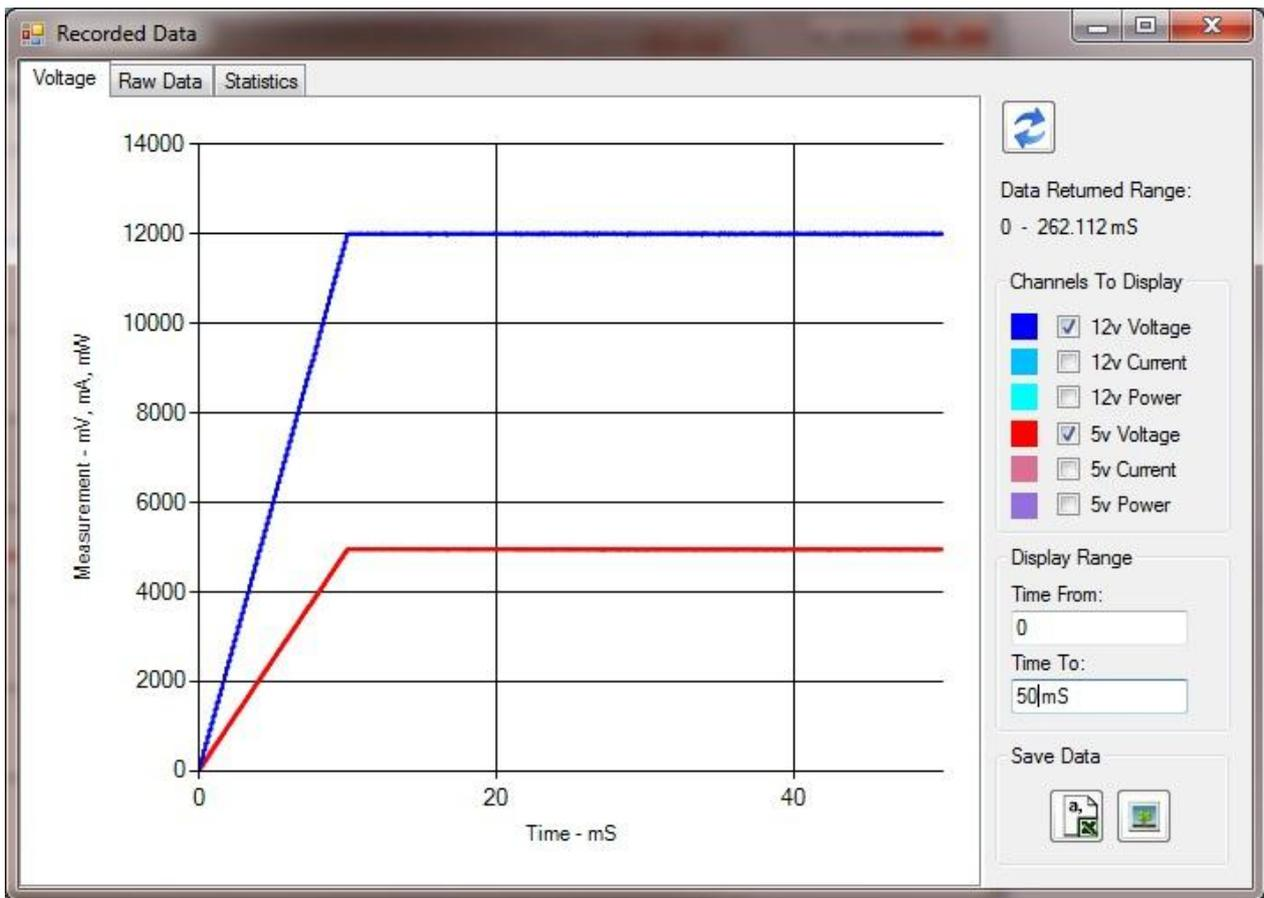
Zooming in to 50mS, we can see that the voltage outputs ramped up exactly as expected and with very little noise
