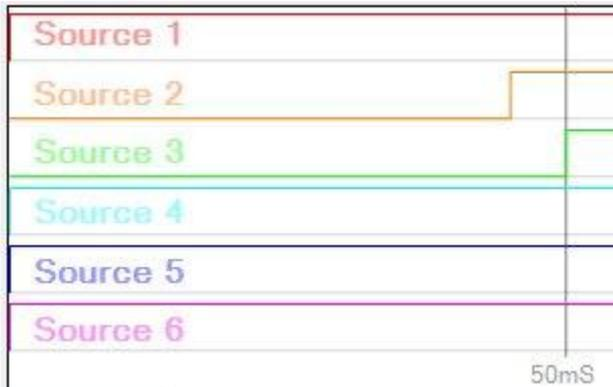
The timing graph shows the new connection sequence with a much shorter time between the connection of Source 2 and Source 3
