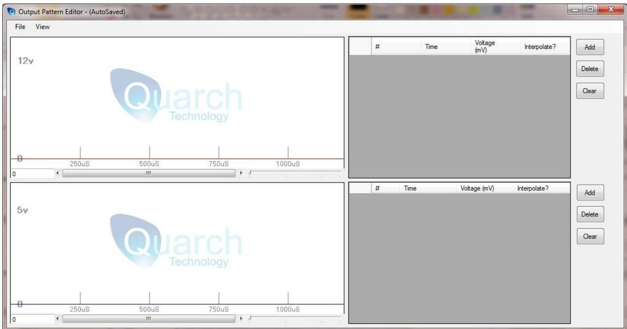
To create a pattern, first set the output voltages to the level you require at the start of the pattern. In this example we set the outputs to 0mV so we can create a ramp. Select **Edit Output Pattern** from the main window, the editor will be displayed as above
