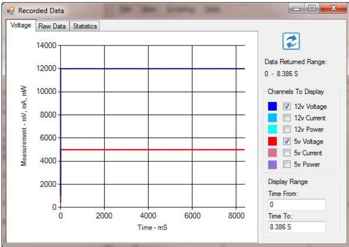
Only the voltage measurement are shown in this example. Check the check boxes to add and remove other items from the graph. If you chose to disable some of the record options on the main screen then you will not be able to display them here, the options will be greyed out.
