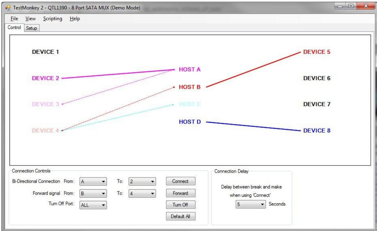
If we use the **Turn Off** port command we will remove the link that goes TO that port. If we turn off Port 4, we will remove the link from **B->4**:
