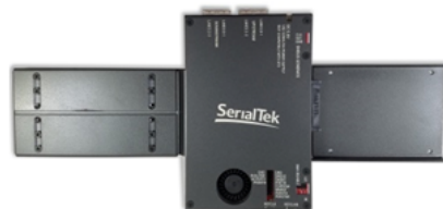
PCIe/NVMe analyzer 的三种 interposer: Slot, U.2, M.2
