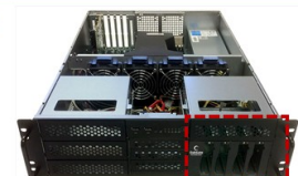
Installed in 3U Rackmount Appliance
