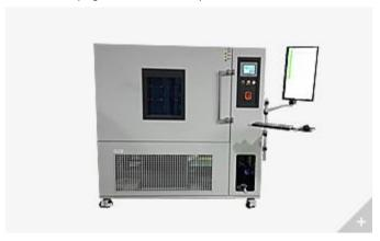
The eMMC Tester II is capable of conducting power-cycle tests under high or low temperature conditions, which simulates a similar testing environment of eMMC device used for in-vehicle devices that operate under extreme temperature. The burn-in test equipment in the test chamber minimizes testing time and maximizes coverage as it allows users to actually reproduce bad blocks in an eMMC in mass that occur during repetitive uses and easily test the management of the eMMC controller against them.
