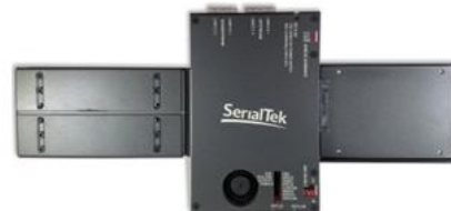
PCIe/NVMe analyzer 的三种 interposer: Slot, U.2, M.2
