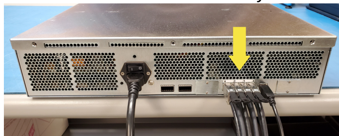
SBExpress-RM5 NVMe SSD Test System populated with cables
