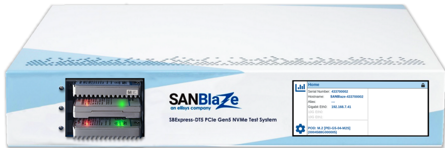
SANBlaze SBExpress-DT5 Gen5 NVMe SSD Test System
